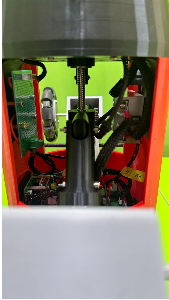
Figure 5.2: Wall Press Mechanism with Lead Screw
