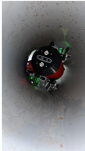
(b) Navigating a 90-degree bend section
